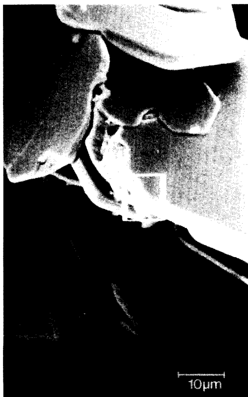
FIG. 4. SEM of oxidized MoS 2 crystals showing reacted edge planes and oxidation pits in the basal plane. Arrow indicates edge plane.
